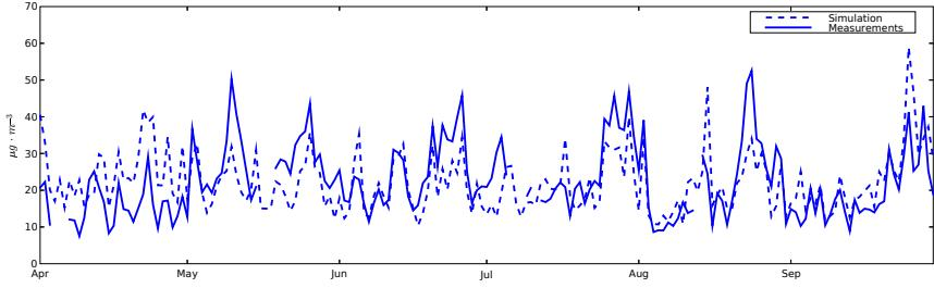
Figure 10: Time series of measured versus simulated  $\text{PM}_{10}$  concentrations at station Gennevilliers (Paris suburb) for April–October 2001.
