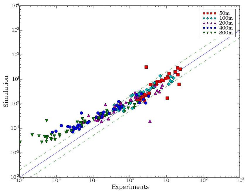
Figure 21: Scatter plot of maximum arc concentrations for observations and simulations with similarity theory parameterization. Prairie Grass experiment, 43 trials. Run with one model configuration of POLYPHEMUS.
