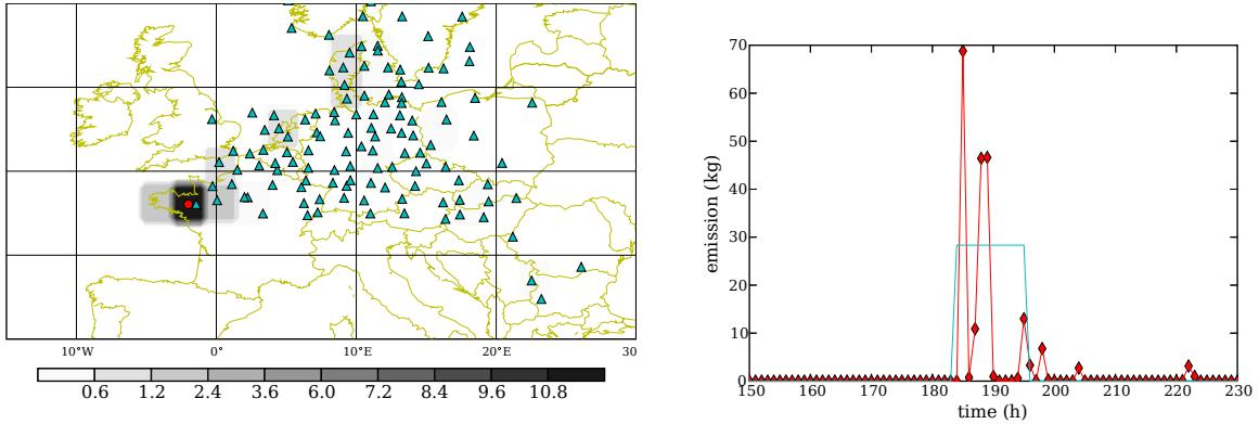
Figure 22: Left: A two-dimensional representation of the reconstructed source of ETEX-I, integrated in time. The inversion is based on the MEM principle. The reconstruction is based on all available positive measurements, the triangles mark the stations whose data were used in this inversion. Right: temporal profile of the solution in the true release grid-cell. 342 kg are recovered (222 kg in the correct grid-cell) against 340 kg known to have been released.
