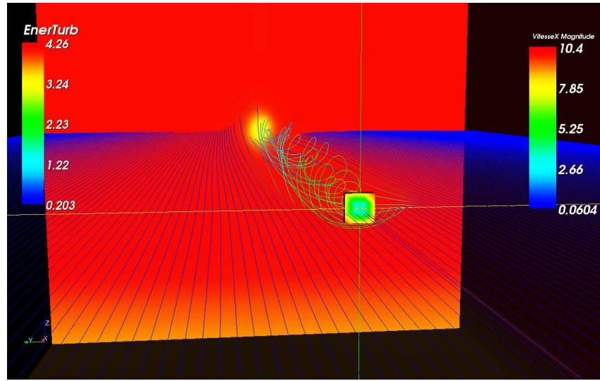
Figure 4: Mercure\_Saturne 3D simulation of a Rutland wind turbine. Stream lines are colored depending on the turbulent kinetic energy. The mesh and the hub are colored according to the wind speed values (Laurent Laporte PhD Thesis).
