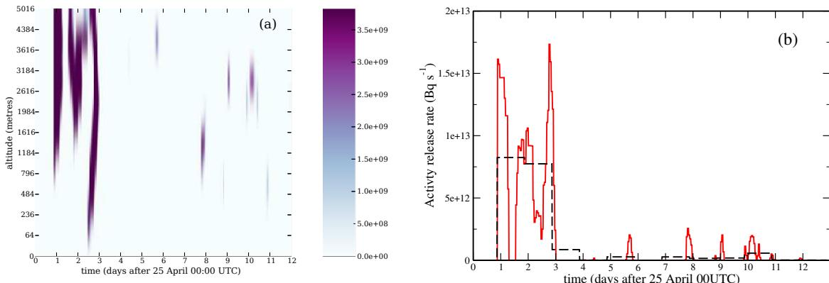
Figure 25: A typical solution of the Chernobyl source inversion problem based on a Bernoulli source prior, and a uniform Gaussian error prior. The left-hand-side figure (a) is a density graph representing the activity released per unit of time and unit of altitude (in  $\text{Bq m}^{-1} \text{s}^{-1}$ ). The right-hand-side figure (b) are reconstructed hourly and day-to-day (dashed line) profiles of the iodine-131 release rate.
