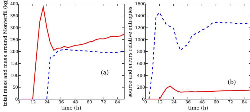
Figure 23: Total PMCH (340 kg were released in ETEX-I in Monterfil) reconstructed mass (full line) and reconstructed mass around Monterfil (dashed line) against time (a). Relative entropy for the source (full line) and relative entropy for the errors (dashed line) against time (b). The time origin corresponds to 23 October 1994 15:00 UTC, one hour before the start of the release.
