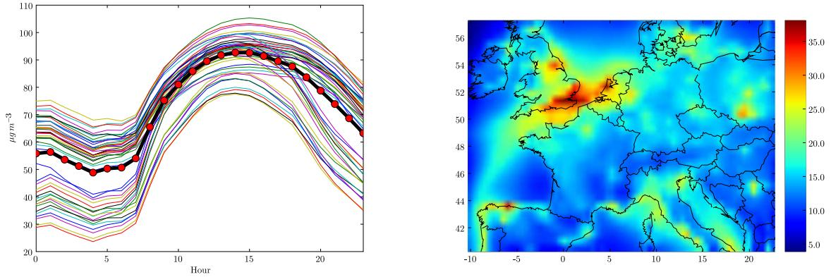
Figure 16: Ensemble forecast with the POLYPHEMUS system (ozone, summer 2001). Left panel: an *ensemble* for hourly profiles of ozone (averaged over Europe and over four months). The points indicate the ensemble forecast. Right panel: ensemble relative variance (in %).
