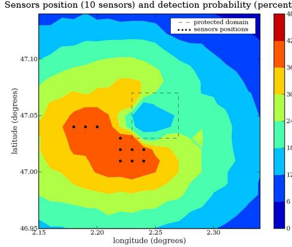
Figure 31: Network design on a battlefield (regional scale). Map of detection probability at regional scale for all possible sensors, as well as the sensors positions for the ten sensors having the best detection probability.
