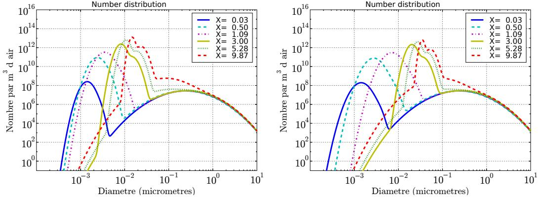
Figure 14: Variation of the number distribution of particles as a function of the distance from the road. The condensation of semi-volatile organics is ignored in the left panel while it is taken into account in the right panel. Bastien Albriet PhD Thesis.
