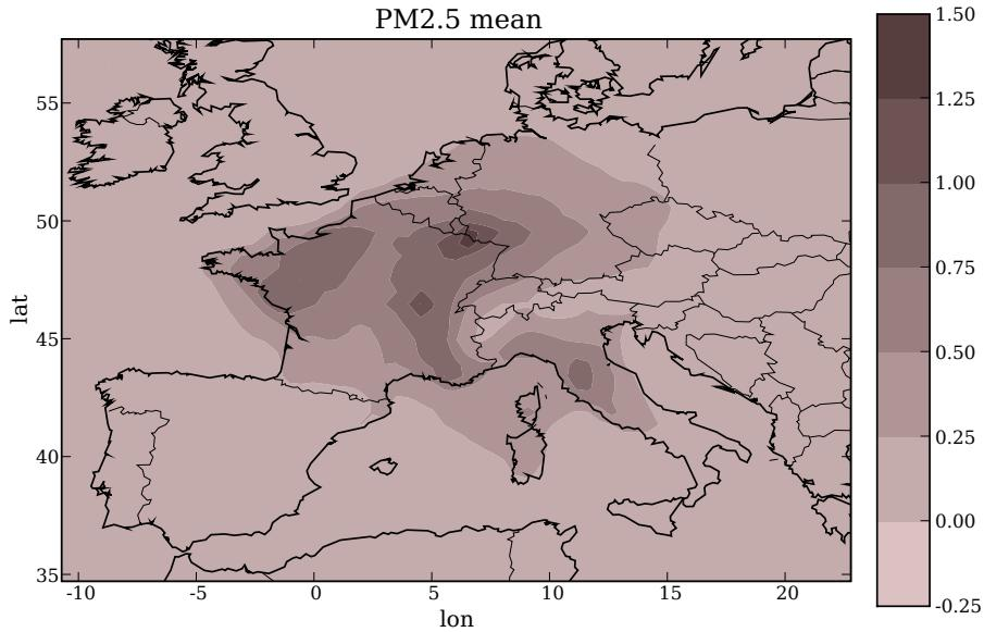
Figure 19: Impact for the year 2005 of the emissions from the French thermal power plants (EDF and SNET). The target is PM<sub>2.5</sub>. The indicator is a relative impact computed in % by comparing a reference simulation and a simulation without the emissions.
