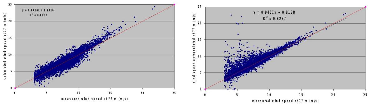
Figure 33: Comparison between computation and measurement of wind speed at 80 m, for a one-year data set (December 2004 to December 2005), with two methods: one using normalized vertical profiles measured by sodar (left panel), one using a simple power law (right panel).
