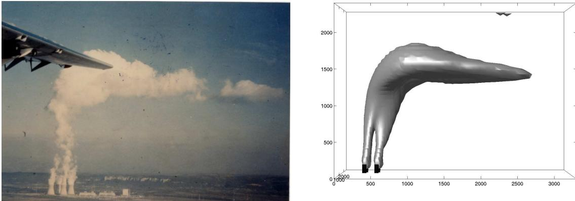
Figure 1: Water droplet plume from cooling towers at the Bugey power plant. Left: plume photograph taken from the measurement airplane. Right: iso-surface of liquid water concentration from numerical simulations using Mercure-Saturne (PhD work of E. Bouzereau).
