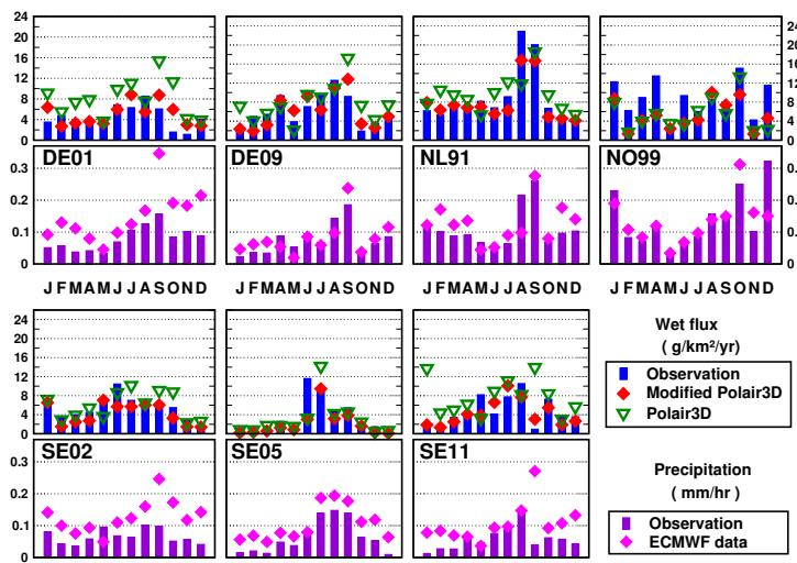
Figure 18: Comparison of model outputs from POLAIR3D and observational data for wet mercury (dissolved in rain droplets). Monthly averaged values in  $\text{g km}^{-2} \text{ yr}^{-1}$ . The modified values are computed with the “right” precipitation fields.
