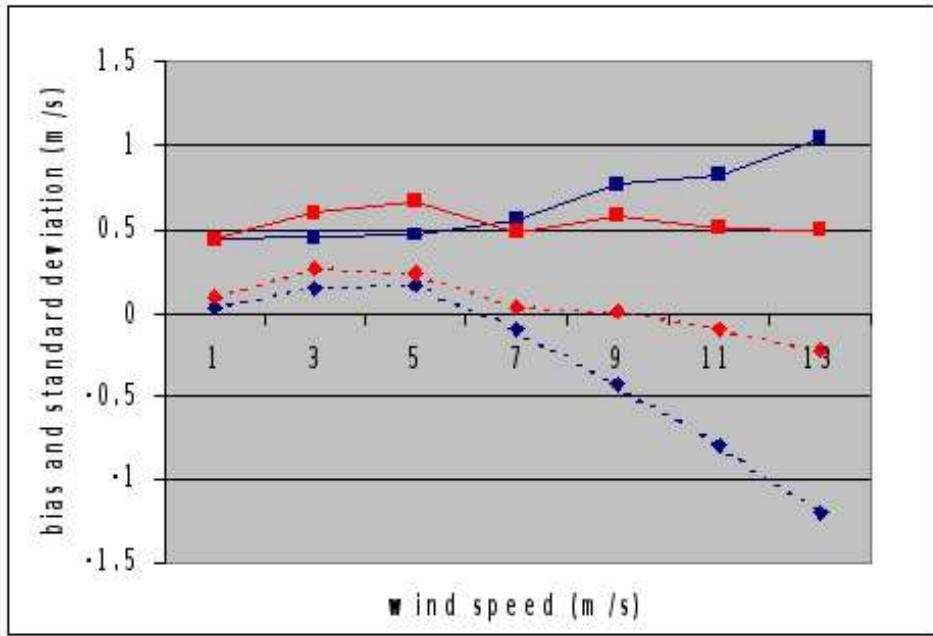
Figure 32: Influence of the wind speed at 80 meters (measured by sonic anemometer) on bias (dotted lines) and standard deviation (solid lines) between sodar and sonic measurements, for 2 of the 3 tested sodars, during the campaign of winter 2005-2006.
